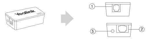
**Port** 1: Connect this port and the IP phone EXT/EHS port or Expansion Module EXT port (the expansion module has been connected to the phone) using the RJ12 cord.
