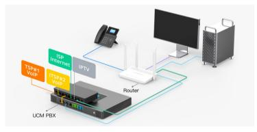
Using VLAN Trunking to merge multiple ITSP streams into a single port connecting to UCM, and merge Internet and IPTV into another port connecting to router and switch.
