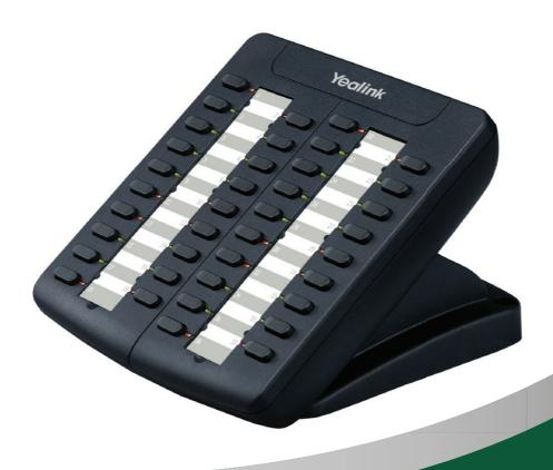
Yealink EXP38 Expansion Module is designed for improving the power and flexibility of Yealink advanced IP phones SIP-T29G/T28P/T27P/T26P. It features 38 fully programmable DSS keys each with a dual-color LED, connected to and controlled by the IP Phone with an RJ-12 cable line. It creates up to 228 additional programmable extensions when 6 EXP38 are daisy chained with the IP Phone.
