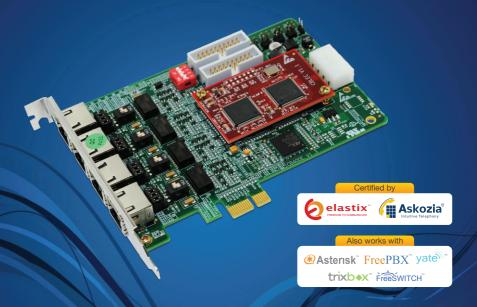
Each of the 4 ports can be independently configured for TE or NT mode
